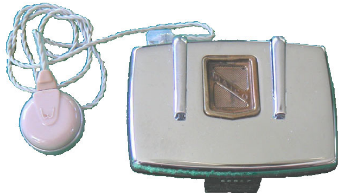
Fig. 22. Maico's Model O "Transist-Ear" was the world's first all-transistor body hearing aid (Jan, 1953).
