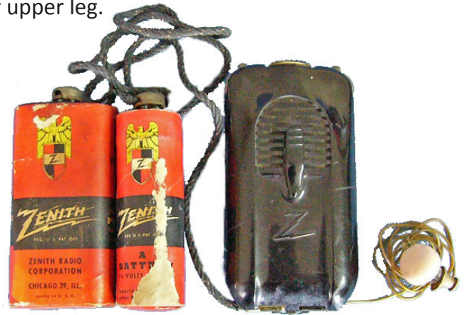
Fig. 18. The Zenith Model A3A-B3A "Radionic"—a two-piece vacuum-tube hearing aid. The large "B" battery is on the left and the round "A" battery beside it (1944).
