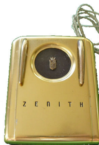
Fig. 23. The Zenith "Royal" vacuum-tube hearing aid was one of Zenith's last vacuum tube hearing aids made (Feb, 1952).
