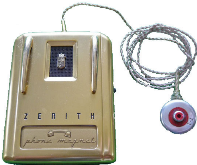
Fig. 24. The Zenith “Royal T” was Zenith’s first all-transistor hearing aid (Feb, 1953). It was the same size as the “Royal” vacuum-tube aid. Note that it had a t-coil built in—called a “phone magnet” in those days.
