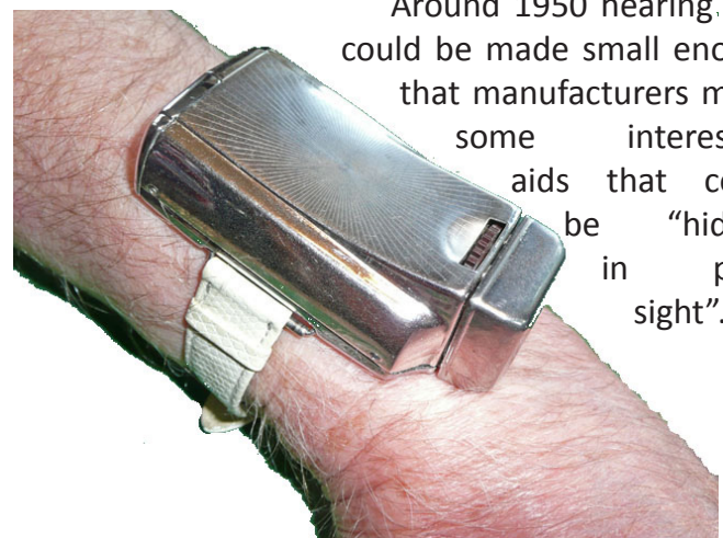
Fig. 19. Acousticon's Model A-165 was the only wrist-worn vacuum-tube hearing aid ever made (1950).
