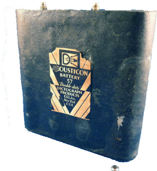
Fig. 29. The Acousticon No. 57 hearing aid battery—one of the largest hearing aid batteries made contrasted with the tiny Panasonic No. 5 battery—the smallest hearing aid battery made.
