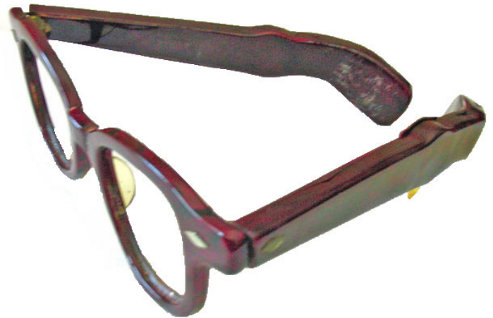
Fig. 27. The Otariion Model L10 “Listener”—the world’s first transistorized, eyeglass hearing aid (Dec, 1954).
