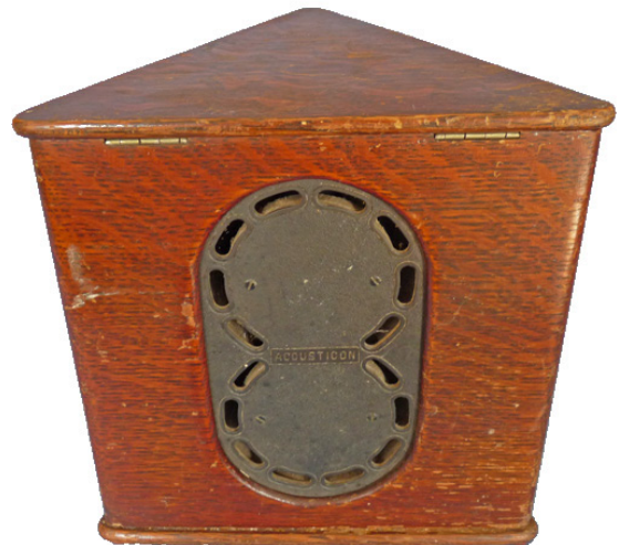
Fig 12. The Acousticon Dining Table Model carbon hearing aid had 6 microphones—2 on each side (1908-1910).
