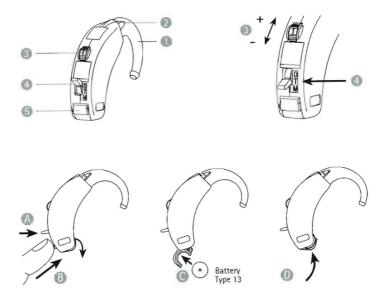
A) Move the M-T-O switch to the "O" (Off) position.
